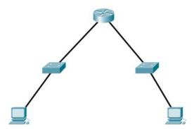
Your task as a network engineer is to configure the subnetwork on the left-hand side with the IPs provided by the first subnet and the subnetwork on the right-hand side with the IPs provided by the second subnet. In the end, both computers shall be able to ping each other.
