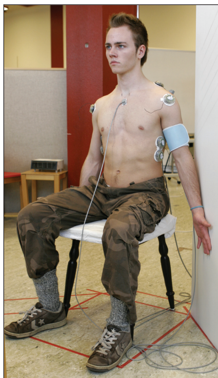
FIGURE 2. Experimental setup. A sensor was attached to the skin of the sternum, to the flat part of the acromion and on the posterior aspect of the humerus. The EMG surface electrodes on the subject were not utilized in this study.
