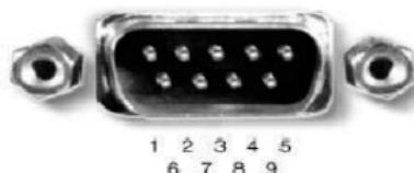
Figura. Porta Serial – Conector DB-9
