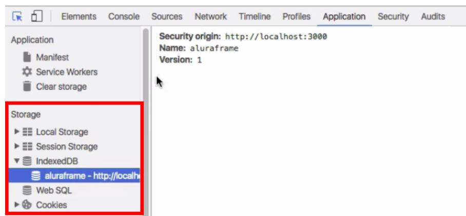
The screenshot shows the Chrome DevTools Application tab. In the left sidebar, under 'Storage', the 'IndexedDB' section is expanded, showing a list of databases. One database is selected: 'aluraframe - http://localhost:3000'. This database entry is highlighted with a red box. The right panel displays details for this database: 'Security origin: http://localhost:3000', 'Name: aluraframe', and 'Version: 1'.
